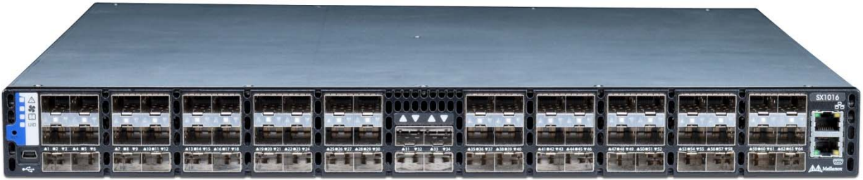
Figure 1: An example of a networking switch with 60 SFP+ ports.
